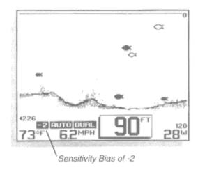
Another use of the Sensitivity menu is to select the bottom representation. The Wide Vision normally displays a variable Structure ID bottom, which can allow experienced users to determine the texture or relative hardness of the bottom. For simplicity, you can select a black bottom using the ENTER button. This blackens in the display below the bottom for easiest recognition of the bottom location, even from a great distance.
